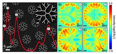
A)SEM image of fourth-order three branched dendritic fractals. Overlaid on the image is the infrared absorption spectrum of the structure. B-E) Finite difference time domain calculations of the electric field distribution at wavelengths corresponding to the numbered resonances.
